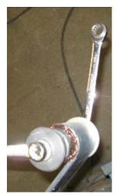
Fit the bearing separator and puller to push the bush in further so it is centrally located in the spring.
